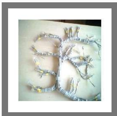
Electric Panel Wiring Harness
